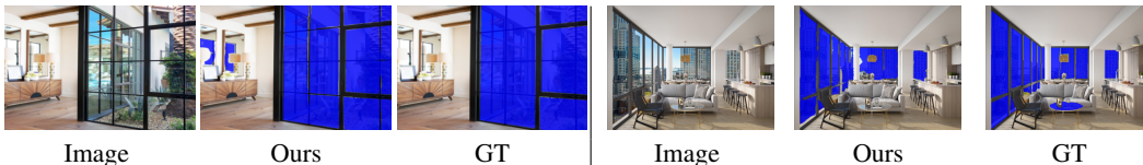
Figure 7: Limitations. Our method may fail to detect glass surfaces in some very challenging scenes with ambiguous visual semantics caused by mirrors or objects of small sizes.
